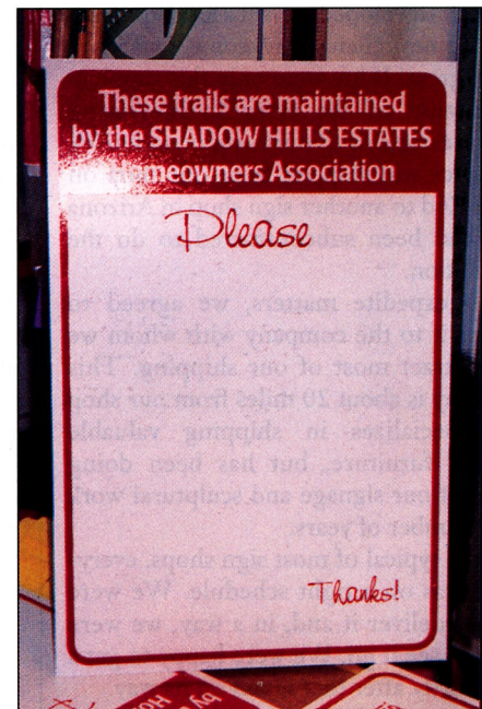
Figure 2: First, I screened the red areas on the sign blanks using enamel ink.
