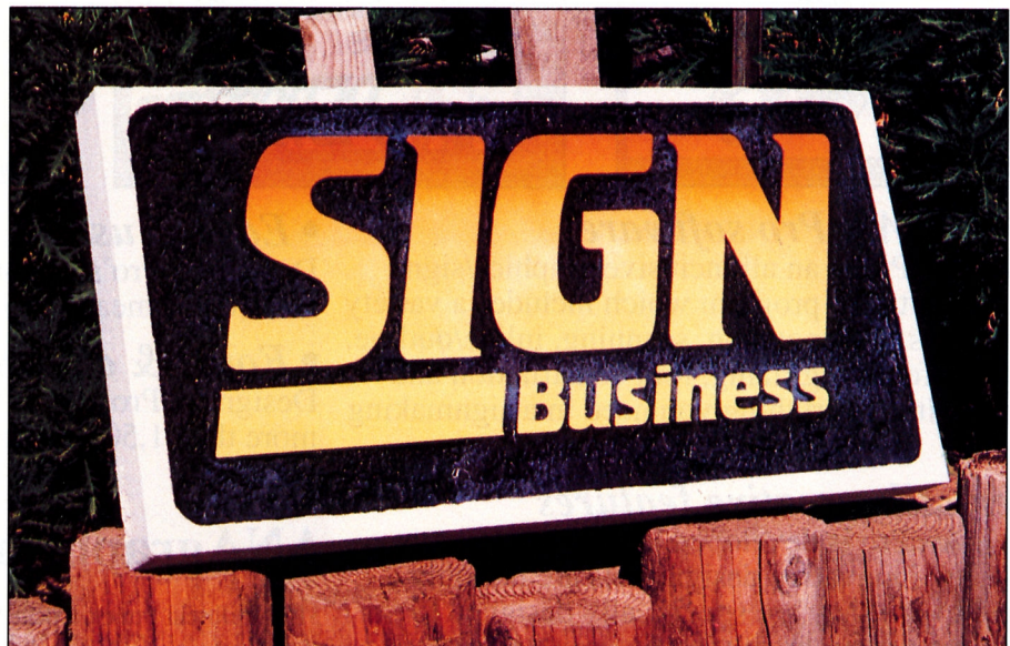
Here's a finished piece, "blasted", painted and airbrushed. The lettering is cut out of vinyl using the original file I created on the computer for the mask with a .05" inline, and stuck on top of the foam for a very clean edge.
