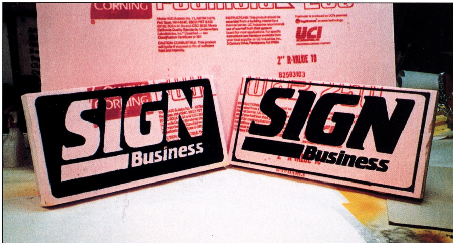
Photo 2: Using flat black Krylon, I lightly coated each blank with numerous coats to get an even "blast", then I removed the paint mask.
