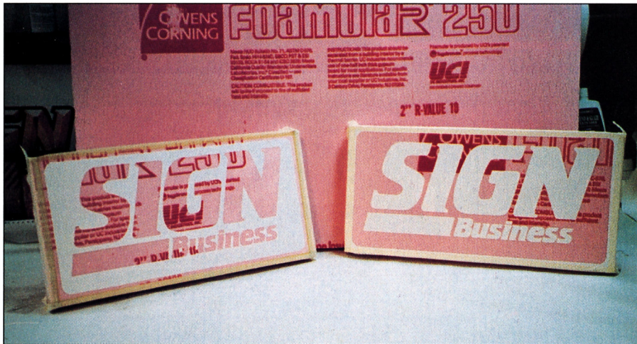
Photo 1: I used paint-mask vinyl in reverse and regular application on two cut-out blanks of Foamular extruded polystyrene insulation. Almost any kind of styrofoam works.
